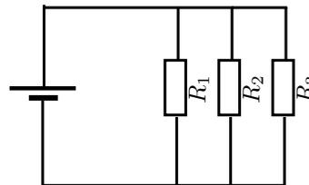
3 resistors in a parallel circuit
