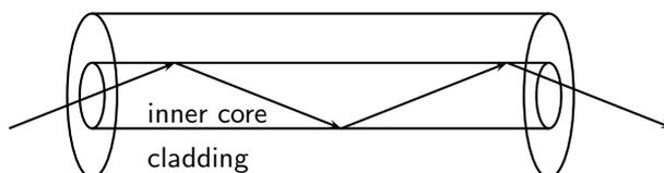
Figure 7.23: Structure of a single optical fibre.
