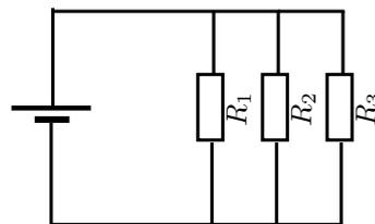
3 resistors in a parallel circuit
