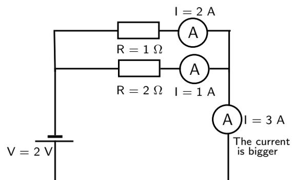
Adding a resistor to the circuit in parallel decreases the total resistance
