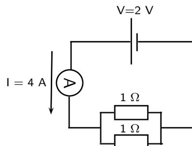
the 2 resistors in parallel result in a *lower* total resistance and therefore a *higher* current in the circuit
