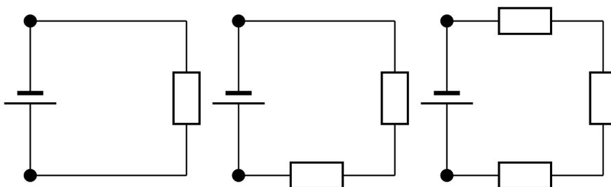
Let us look at this in a bit more detail. In the picture below you can see what the different measurements for 3 identical resistors in series could look like. The total voltage across all three resistors is the sum of the voltages across the individual resistors.
