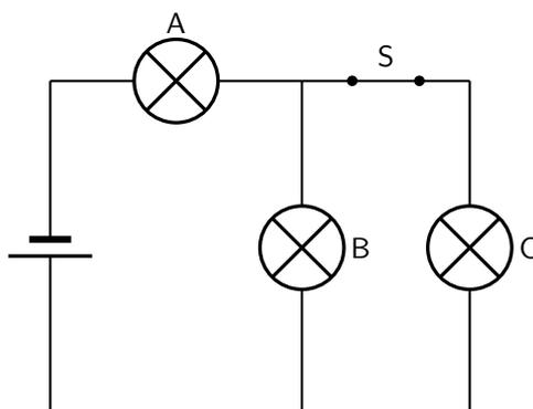
How do the currents in bulbs A and B change when switch S is opened?
