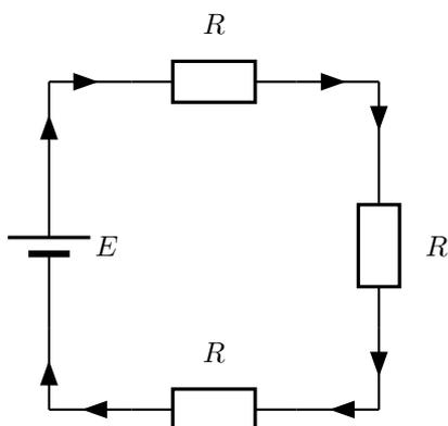
The arrows in this picture show you the direction that charge will flow in the circuit. They don't show you much charge will flow, only the direction.
