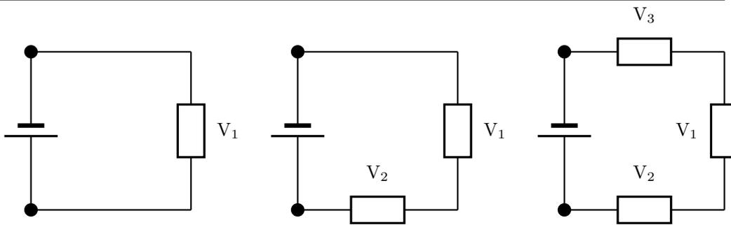
We know that the total voltage is equal to  $V_1$  in the first circuit, to  $V_1 + V_2$  in the second circuit and  $V_1 + V_2 + V_3$  in the third circuit.
