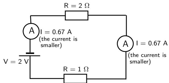
Adding a resistor to the circuit increases the total resistance
