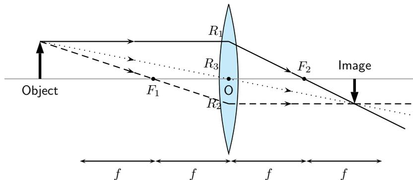
Figure 13.7: An object is placed at a distance greater than  $2f$  away from the converging lens. Three rays are drawn to locate the image, which is real, smaller than the object and inverted.
