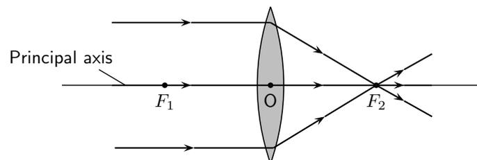
Figure 13.5: Light rays bend towards each other or *converge* when they travel through a convex lens.  $F_1$  and  $F_2$  are the foci of the lens.
