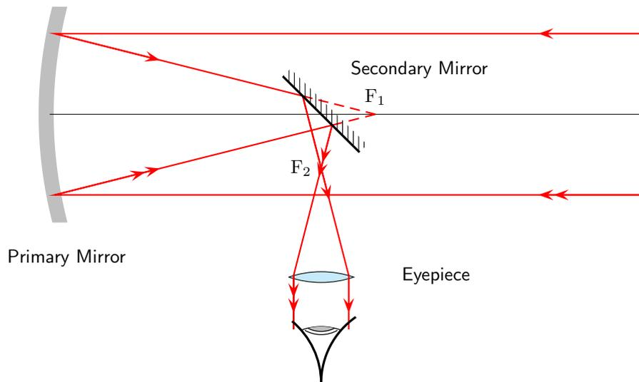
Figure 13.21: Lenses and mirrors in a reflecting telescope.
